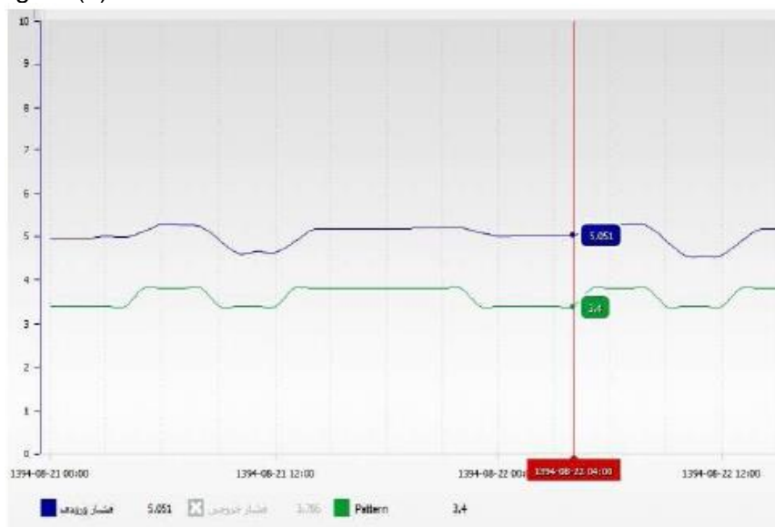
Fig(3) minimum out put pressure of pressure reducing valve at night
